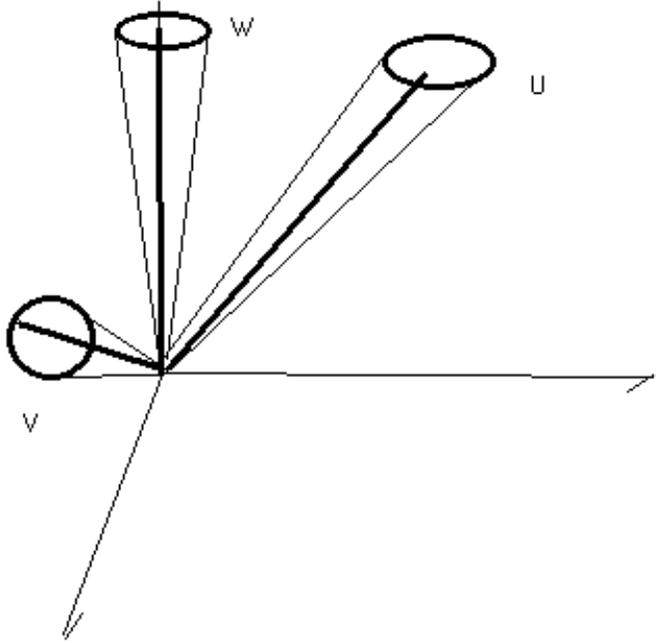
**Figure 1 Idealized acoustic beam pattern from a 3-beam sodar.**
