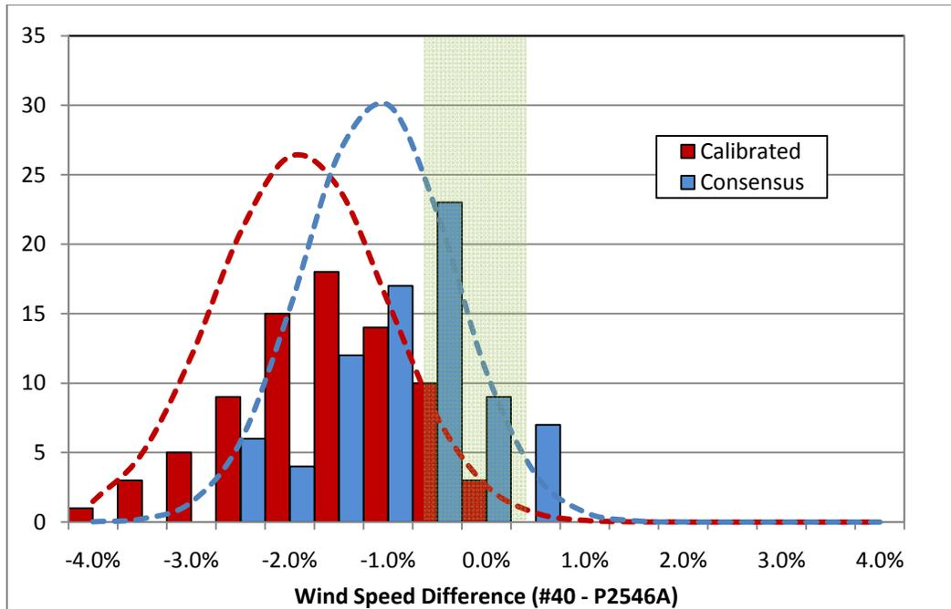
**Figure 1. Comparison of differences in mean wind speed between NRG #40 and WindSensor P2546A anemometers using the NRG #40 calibrated and consensus transfer functions.**
