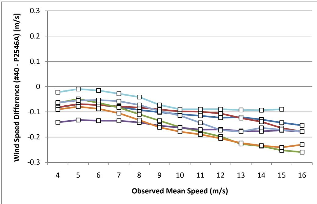
Figure 2. Mean biases of a sample of anemometer pairs in seven unique geographical locations using calibrated transfer functions. A clear downward trend with wind speed exists at six of the seven sites.
