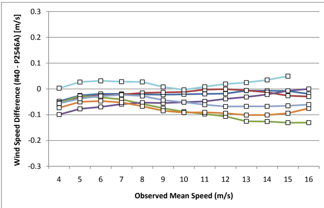
Figure 3. Mean biases of a sample of anemometer pairs in seven unique geographical locations using the consensus transfer function. There is generally a flat trend vs. wind speed.
