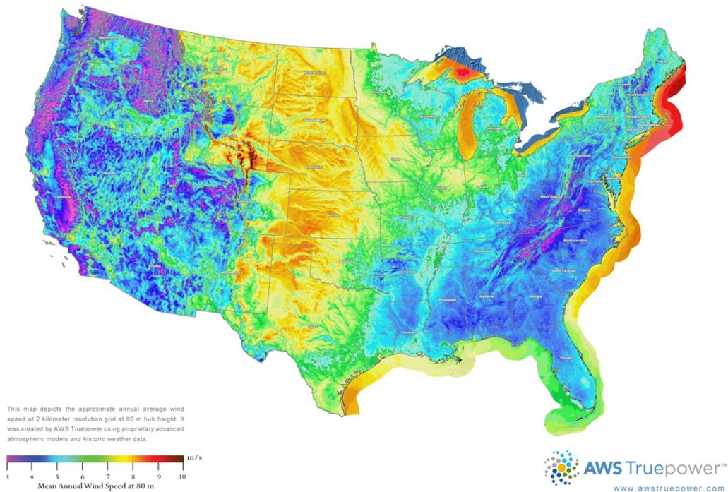
**Figure.** Wind Resource Map of United States created with MesoMap® system by AWS Truepower.
