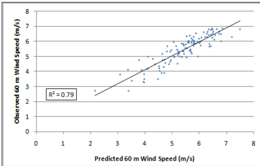
Figure 4. Modeled versus observed annual mean wind speeds at 60 m hub height
