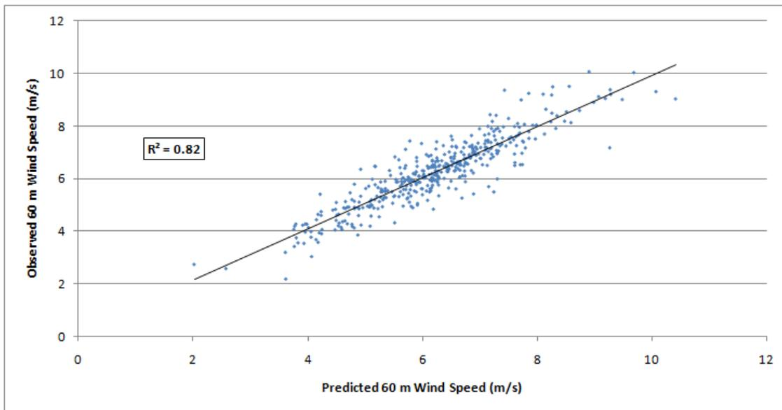
Figure 5. Modeled versus observed annual mean wind speeds at 60 m hub height
